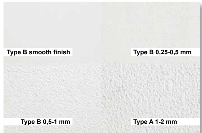
Grain size of the various finishes
